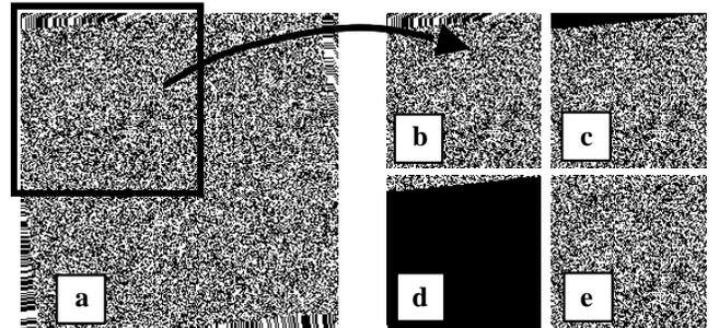
**Figure 3.** (a),(b) noise texture advected by a circular flow  $(u, v) = (-y, x)$ . (c) regions from particles exterior to the domain at the previous step are black ( $I_1$ ). (d) new noise is injected into the edge region; complement region is black ( $I_2$ ). (e) composite of  $I_1$  and  $I_2$ .
