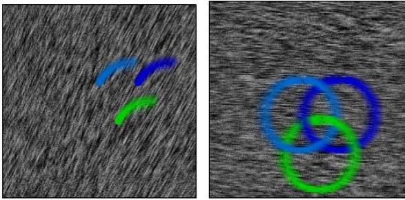
**Figure 7.** Three streaklines in the rotating uniform flow  $(u,v) = (\cos(t), \sin(t))$  (see [5]).
