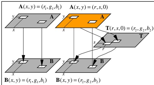
**Figure 1.** Pixel Texture. (left) Color triplets are transferred directly to the framebuffer. (right) When a pixel texture is applied, color triplets are used to address its texels, whose values are sent to the framebuffer.
