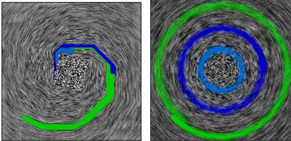
**Figure 5.** Dye advection in a circular flow defined by the circular flow  $(u, v) = (-y, x)$ . Left: fractional coordinate correction is disabled. Right: fractional correction is enabled.
