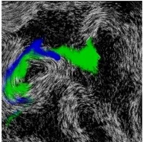
**Figure 8.** Two frames from a 1000 frame animation (computed in 11 minutes) sequence of wind currents over Europe [17]. Note the lack of artifacts at the domain boundaries. Dye is released from a point and from a line segment. Vortical patterns are evident in the lower frame.
