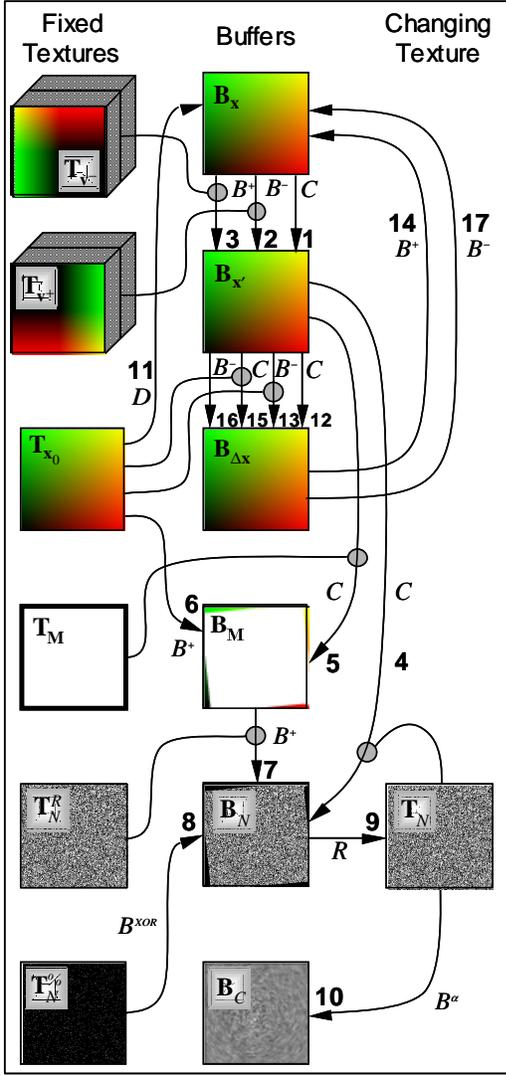
**Figure 2.** Algorithm for a single time step. The numbers indicate the operation number in the algorithm, which matches the line number in table 1. Pixel texture operations are shown as circles.
